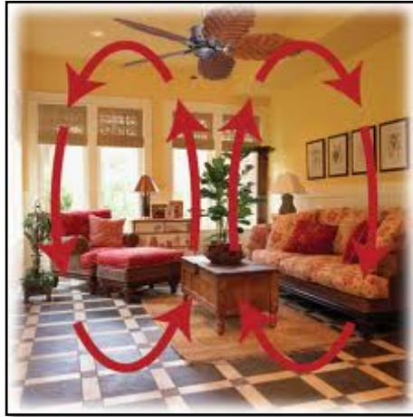
Figure 26: Ceiling fan circulating warm air in winter
